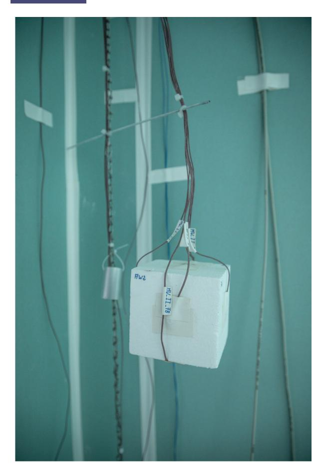
As part of the trial, the researchers collected a large amount of indoor climate data, which they then used to validate the digital twin. Credit: Fraunhofer-Gesellschaft
