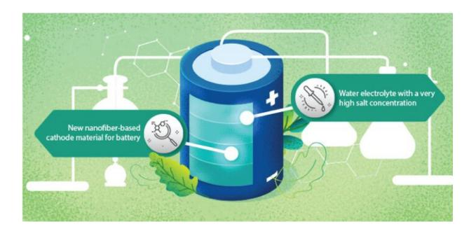
A new electrolyte and electrode combination can improve zinc-ion battery performance, which may make zinc-ion batteries more attractive than their lithium-ion counterparts. Credit: KAUST; Veronica Moraru
