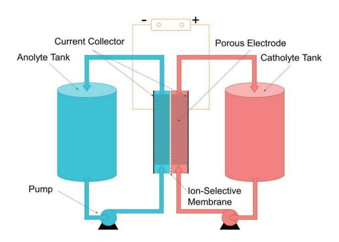
A typical flow battery consists of two tanks of liquids that are pumped past a membrane held between two electrodes. Credit: Qi and Koenig, 2017, CC BY
