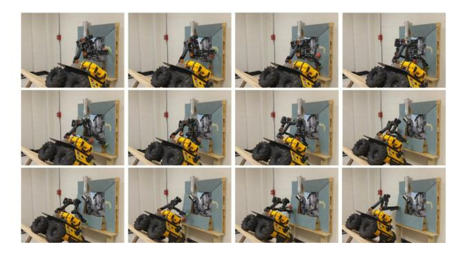
A two-arm mobile manipulator, which would fall if it did not brace itself on the wall, rolls across the steep incline by using the team's approach to identify placements for its arms. Credit: Yu-Chi Lin.
