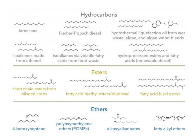
The 13 top-performing blendstocks with the potential to reduce criteria and GHG emissions comprise 6 hydrocarbons, 3 esters, and 4 ethers. Credit: Dan Gaspar, Pacific Northwest National Laboratory
