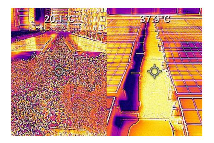
Surface temperatures were up to 20 degrees lower on the green roof compared with the standard solar roof on hot days. Image: UTS research team. Credit: University of Technology, Sydney
