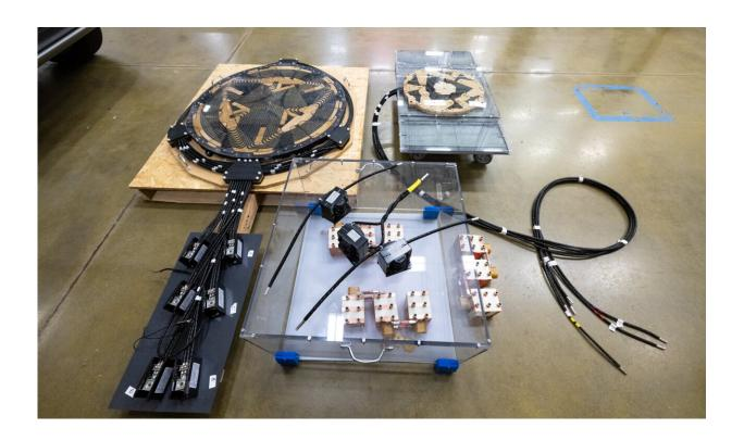
ORNL has licensed its high-powered wireless vehicle charging technology to HEVO, including the lab's unique, compact polyphase electromagnetic coils that provide the highest surface power density available. Credit: Carlos Jones, Oak Ridge National Laboratory/U.S. Dept. of Energy
