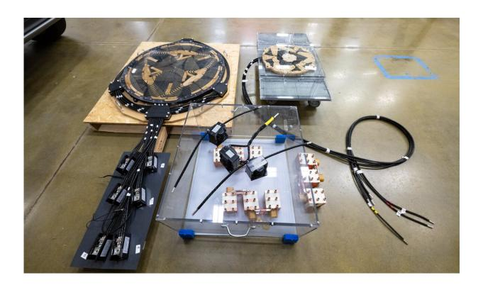
ORNL has licensed its high-powered wireless vehicle charging technology to HEVO, including the lab's unique, compact polyphase electromagnetic coils that provide the highest surface power density available. Credit: Carlos Jones, Oak Ridge National Laboratory/U.S. Dept. of Energy
