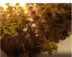
Initial growth stage (left) and later growth stage of the "pre-harvested" lichen blocks on a 3D printed cork lattice for air detoxification reactivity maximization. Credit: University of California - Berkeley
