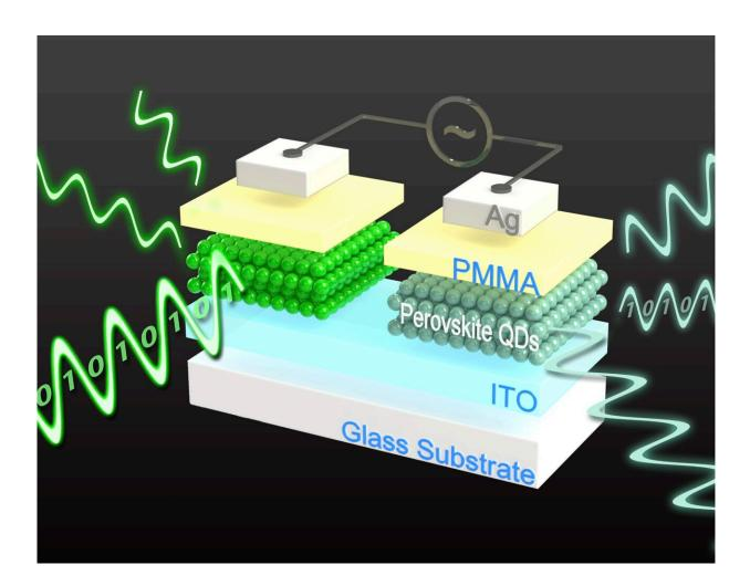
An artist's rendering shows the capability of a CsPbBr<sub>3</sub> LEM device for parallel optical and electrical transmission of encoded information. Two colors can be emitted by the perovskite LEM: green and aqua. These two colors could serve as a real-time indicator of the digital status i.e., write or erase of the LEM. Researchers have shown that such seamless integration of photonic emission and
