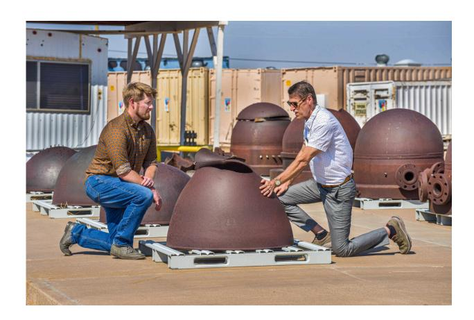
Brad Beeny, left, a Sandia National Laboratories nuclear engineer and code developer, and Larry Humphries, the lead code developer for Sandia's nuclear accident modeling computer code, examine remnants from a series of Lower Head Failure experiments. The results from these experiments, and many others, are used to inform the code. Credit: Randy Montoya
