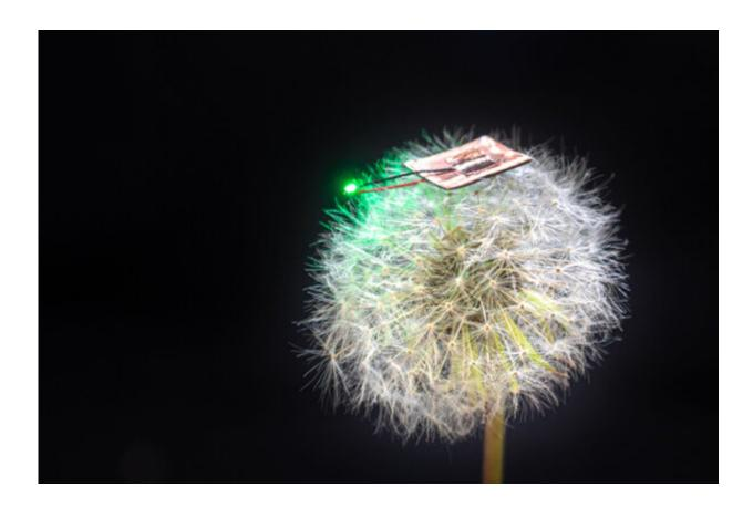
Weighing about as much as two grains of rice but with the energy density of a much larger, heavier battery, the researchers' packing-free design could enable a host of otherwise impossible electronics. Credit: Penn Engineering Today
