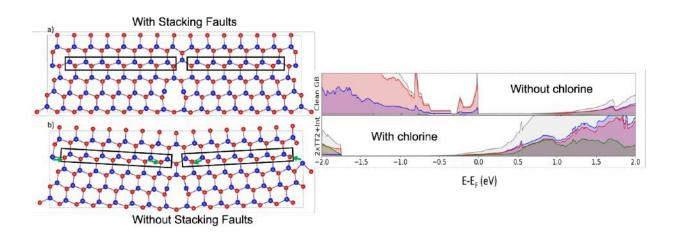
Left: CdTe model with and without stacking faults. Right: Electronic properties showing the removal of mid-gap defect peaks with chlorine (passivation of grain boundaries), which improves efficiency. Credit: Loughborough University
