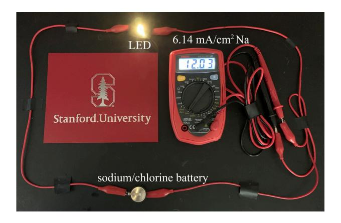
An LED light powered by a prototype rechargeable battery using the sodiumchlorine chemistry developed recently by researchers at Stanford University. Credit: Guanzhou Zhu
