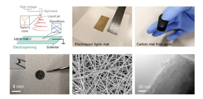
The electrospinning of lignin nanofibres and the structure of obtained carbon mats. Credit: Zhen Xu/Imperial College London
