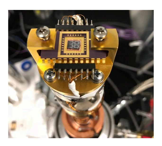
Silicon nanowire prototype being prepared for property measurements in a cryostat. Credit: Lin Yang, Berkeley Lab
