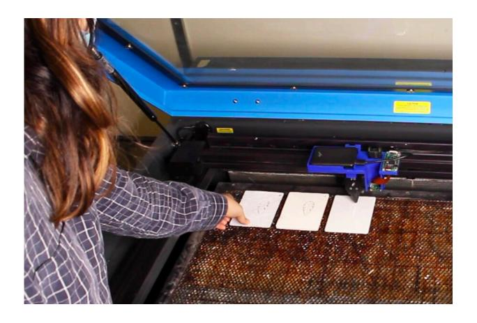
Caption: The SensiCut smart sensing platform distinguishes between visually similar materials for safe use. Credit: MIT CSAIL
