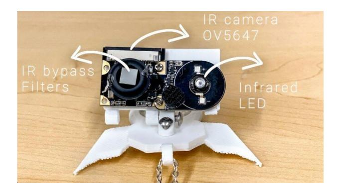
A close-up of the NeckFace wearable sensing technology hardware, which includes an infrared camera, a near-infrared LED and an IR narrow band-pass filter. Credit: Sci-Fi Lab/Provided
