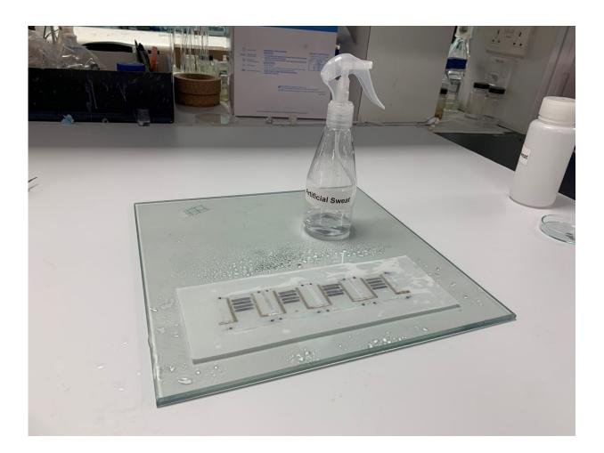
To demonstrate its potential use when it becomes incorporated in wearable biosensors and other electronic devices, the team of scientists at NTU tested their device with artificial human sweat. Credit: Nanyang Technological University
