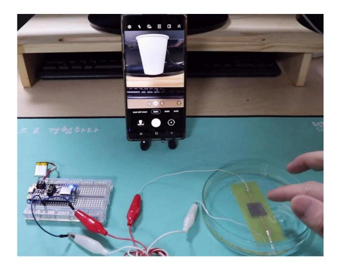
Scientists in Korea have developed a pressure sensor that can control a cell phone from underwater. Credit: Science and Technology of Advanced Materials
