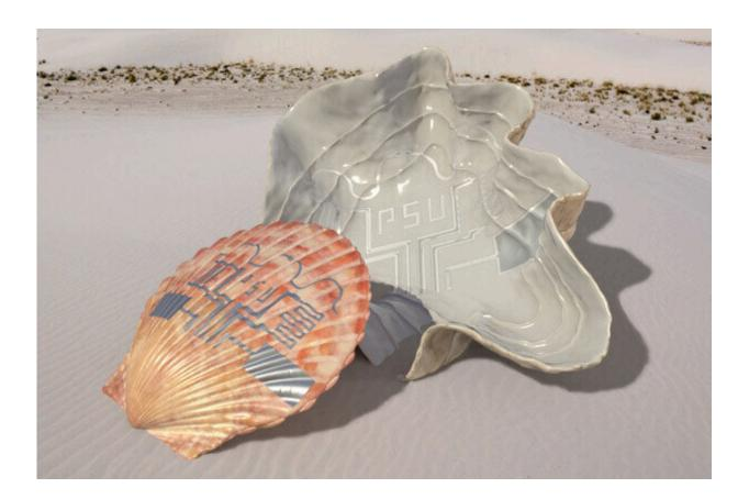
Led by Penn State, an international team of researchers demonstrated a new printing method using pulsed light to transfer an electronic circuit to a seashell, as depicted in this illustration. Credit: Jennifer McCann / Penn State
