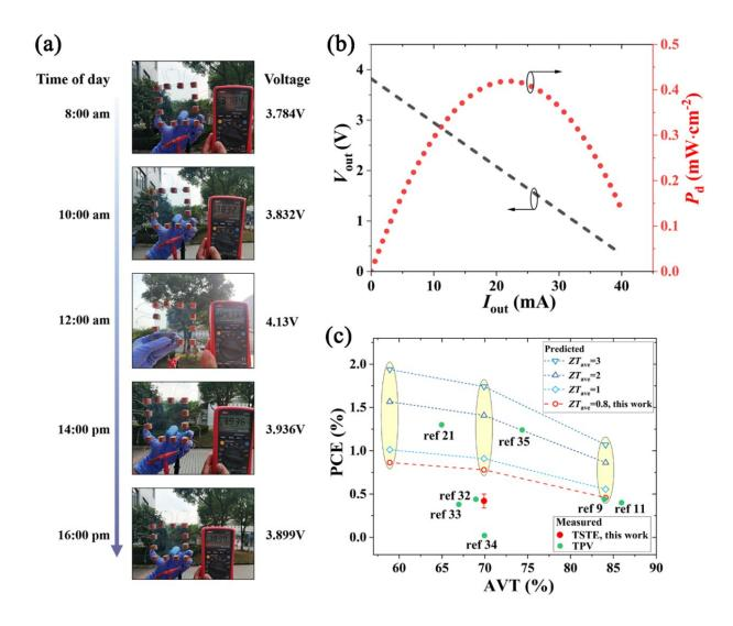
Fig. 2 Power-generating performance of a typical solar-thermal-electric power-generating window. Credit: SICCAS
