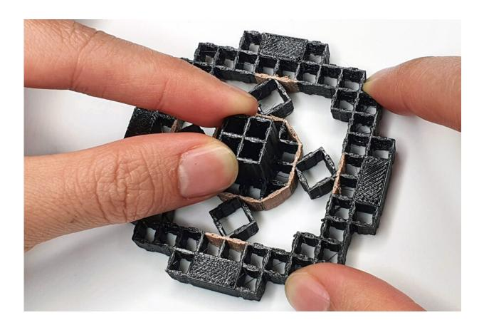
Researchers from MIT have developed a method to integrate sensing capabilities into 3D printable structures comprised of repetitive cells, which enables designers to rapidly prototype interactive input devices. Credit: Massachusetts Institute of Technology
