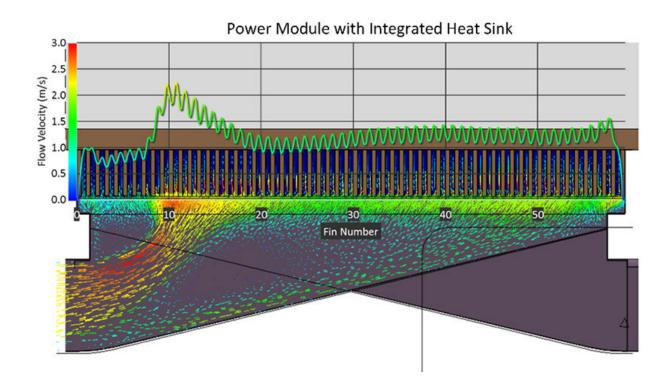
NREL's integrated thermal management system incorporates perpendicular jet flow to extract heat from the system. Credit: Emily Cousineau, NREL
