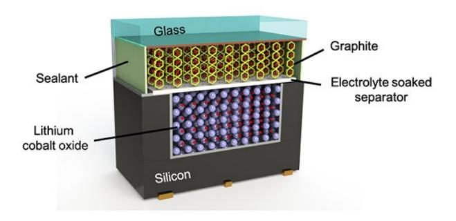
Microbattery fabricated on the backside of a Si chip by stencil printing Lithium cobalt oxide (LCO) in a cavity in Si followed by assembly and bonding with a glass substrate with a printed graphite layer. Credit: University of California - Berkeley
