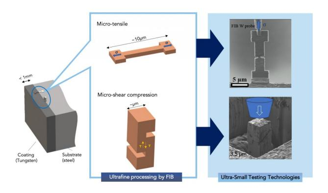
The evaluation flow of direct of interfacial strength by ultra-small testing technology. Credit: Wu Xiangyu
