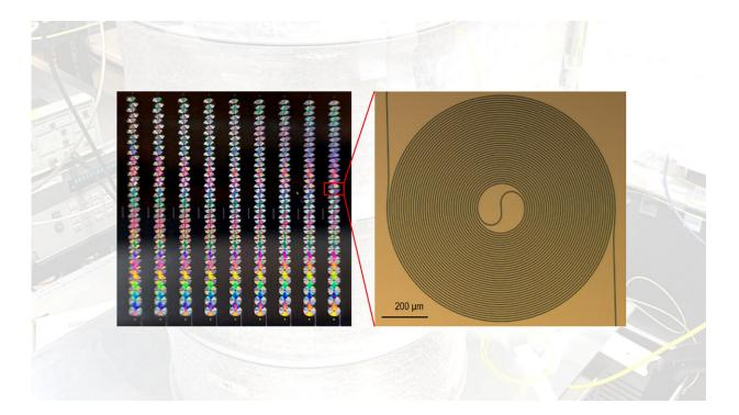
The new component is made of silicon nitride and consists of nine separate waveguides (left). Each waveguide is composed of 22 spirals and can amplify light by about ten times with a noise figure of only 1.2 decibels. Each spiral (right) has an area of 1 square millimeter and the shape enables the compact design of the amplifier. Credit: Zhichao Ye and Yen Strandqvist/Chalmers University of Technology
