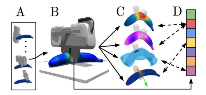
DefGraspSim contributes a pipeline and dataset where (A) For any set of candidate grasps on a deformable object, (B) one can simulate the object's response with FEM, (C) measure the performance metrics (e.g., stress, deformation, instability, deformation controllability), and (D) measure customizable pre-pickup grasp features. The team's simulated dataset contains 34 objects, 6800 grasp evaluations, and 1.1 M unique measurements. Credit: Huang et al.
