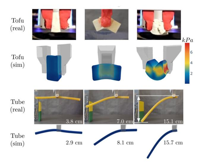
There is good correspondence between the researchers' simulated and real-world experiments, as seen in examples of 3 different grasps on a real and simulated block of tofu (top 2 rows), and 3 different grasps on a real and simulated latex tube (bottom 2 rows). Credit: Huang et al.
