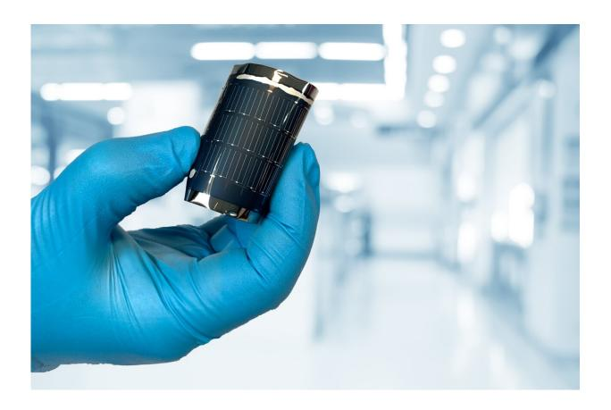
CIGS flexible solar cells consist of very thin layers and include a compound composed of the elements copper, indium, gallium and selenium. The layers are deposited onto flexible polymer substrates, mainly by vacuum processes. Credit: Empa
