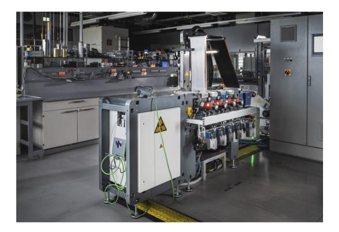
DRYtraec machines do not require long drying tracks and so take up significantly less space than conventional battery electrode manufacturing systems. Credit: Fraunhofer-Gesellschaft
