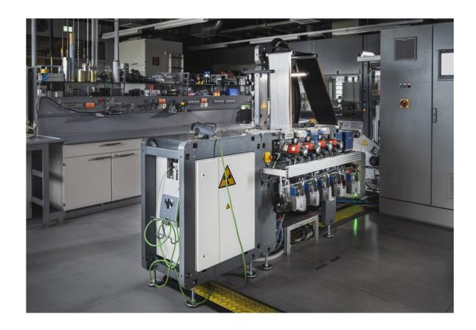
DRYtraec machines do not require long drying tracks and so take up significantly less space than conventional battery electrode manufacturing systems. Credit: Fraunhofer-Gesellschaft
