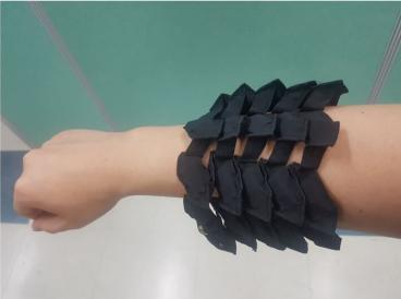
The flexible, stretchable battery developed by the research team of Dr. Bongkyun Jang and Dr. Seungmin Hyun at the KIMM Department of Nano-Mechanics is shown on an individual's arm and hand. The battery is not only capable of conformably attaching to the shape of the human body, but can also morph freely to match the wearer's movement. Credit: Korea Institute of Machinery and Materials (KIMM)
