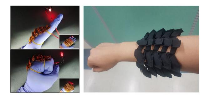
The flexible, stretchable battery developed by the research team of Dr. Bongkyun Jang and Dr. Seungmin Hyun at the KIMM Department of Nano-Mechanics is shown on an individual's arm and hand. The battery is not only capable of conformably attaching to the shape of the human body, but can also morph freely to match the wearer's movement. Credit: Korea Institute of Machinery and Materials (KIMM)
