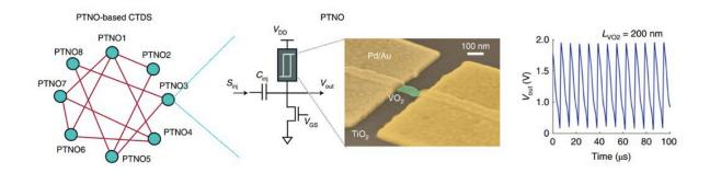
Network of coupled PTNOs fabricated using a complex correlated oxide insulator (Vanadium dioxide VO2) that shows abrupt insulator to metal phase-transition. Credit: Dutta et al.
