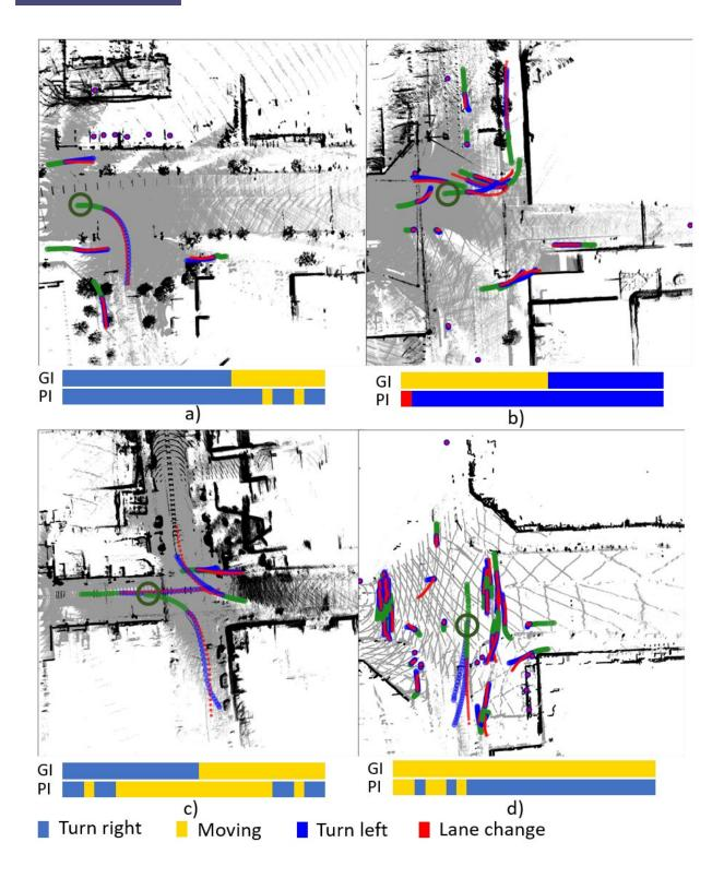
Visualization of top-1 trajectory prediction result (green: past observation, blue: ground truth, red: prediction) and frame-wise intention of a particular agent in dark green circle at the start of the observation time step (GI: Ground truth
