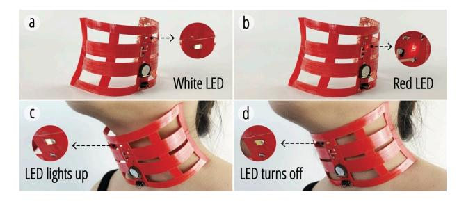
LED indicators indicate when temperature is at a safe handling temperature and tightness of fit.
