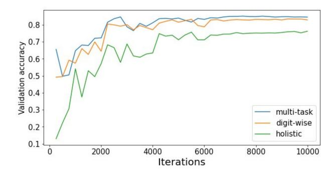
Validation accuracy vs number of iterations for the multi-task learning(MTL), holistic and digit-wise loss settings. The multi-task setting shows the best performance among the three settings. Credit: Vats et al.
