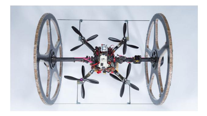
Team CoSTAR's Rollocopter uses a quadrotor system to fly or roll along on two passive wheels. When it meets an obstacle while rolling, it can simply fly over it. Credit: NASA/JPL-Caltech
