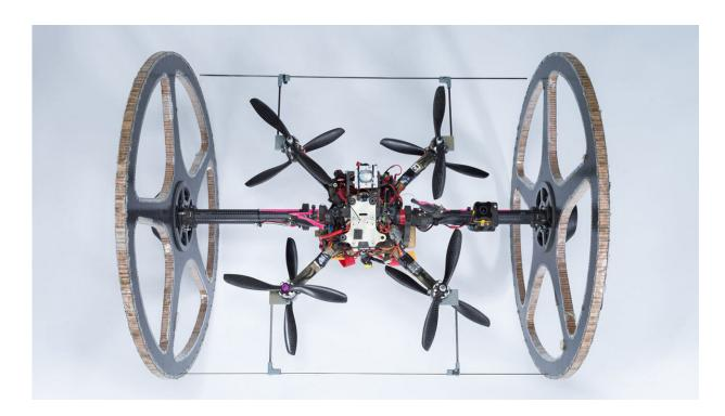
Team CoSTAR's Rollocopter uses a quadrotor system to fly or roll along on two passive wheels. When it meets an obstacle while rolling, it can simply fly over it. Credit: NASA/JPL-Caltech
