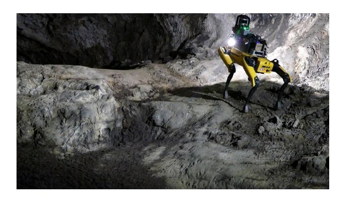
Team CoSTAR, led by NASA's JPL, will use autonomous robots with diverse methods of movement to compete in the complex underground environments of the SubT Challenge Final. One of the robots, <a href="NeBula-Spot">NeBula-Spot</a>, walks on four legs to explore hard-to-access locations. Credit: NASA/JPL-Caltech
