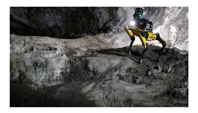
Team CoSTAR, led by NASA's JPL, will use autonomous robots with diverse methods of movement to compete in the complex underground environments of the SubT Challenge Final. One of the robots, <u>NeBula-Spot</u>, walks on four legs to explore hard-to-access locations. Credit: NASA/JPL-Caltech
