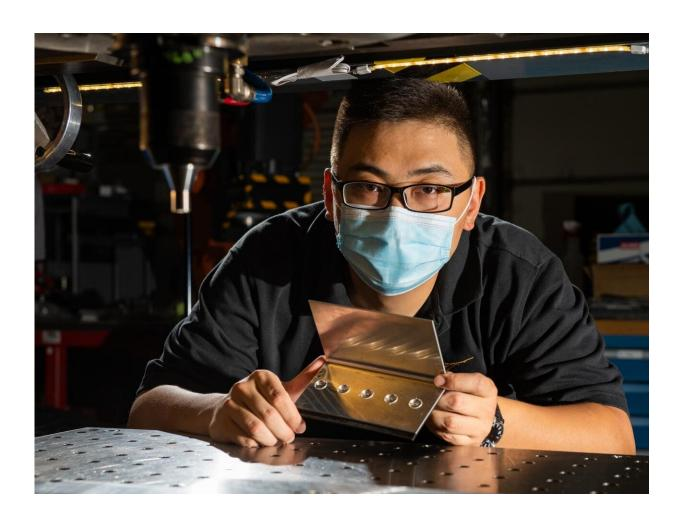
PNNL's new Rotating Hammer Riveting technology enables lightweight magnesium rivets to be used without preheating the rivets. The process is also faster than conventional riveting. Credit: Andrea Starr | Pacific Northwest National Laboratory
