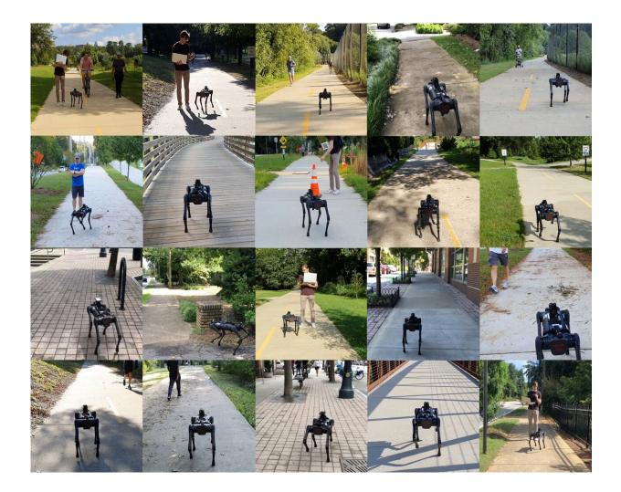
Robot autonomously navigating various real-world sidewalks outdoors in the real
