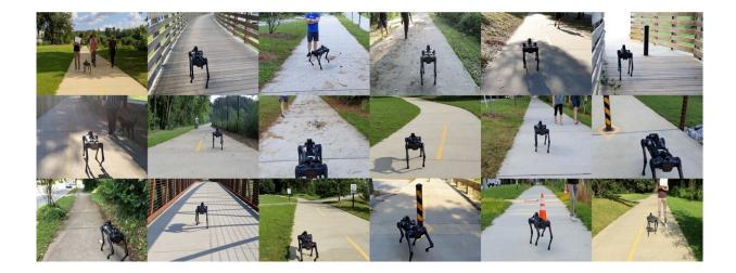
Robot autonomously navigating various real-world sidewalks outdoors in the real world. Credit: Sorokin et al.
