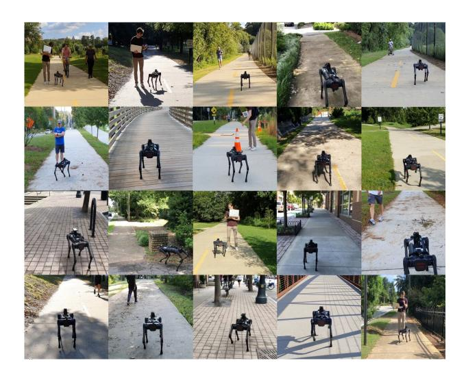
Robot autonomously navigating various real-world sidewalks outdoors in the real
