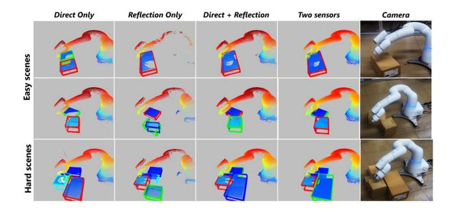
Sensing and detection results are shown with several sensing setups. The researchers' system (Direct+Reflection) can significantly reduce occlusions and misdetections. The sensing results are similar to those achieved when using two sensors in the scene. Credit: Yoshioka et al.
