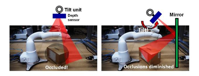
The concept of our tilt-based reflection sensing system. Credit: Yoshioka et al.
