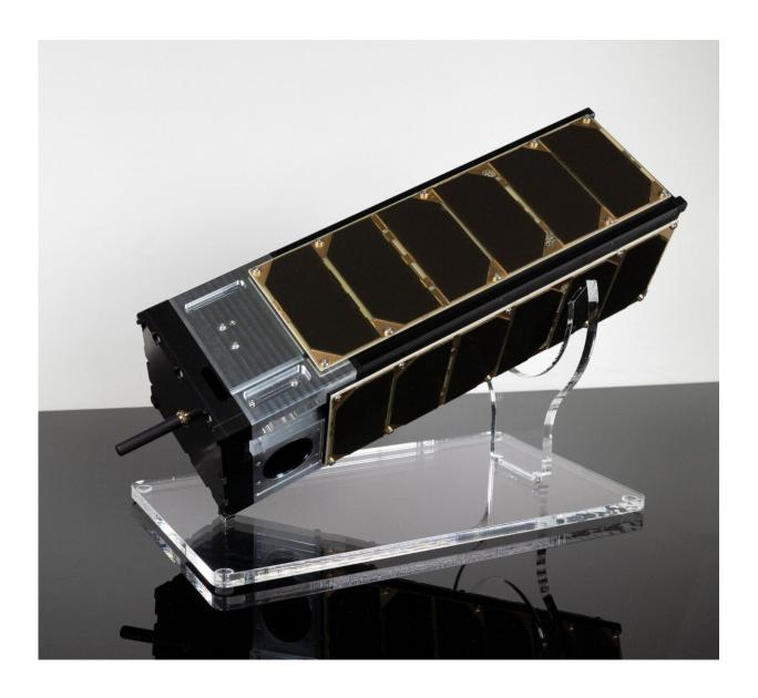
The W-Cube nanosatellite transmits test signals at an altitude of 500 kilometers in the Q and W band (37.5 and 75 GHz) in order to explore new frequencies for
