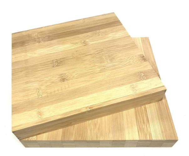
In a similar way to wood, bamboo can be used to manufacture sturdy panels. Credit: Fraunhofer-Gesellschaft
