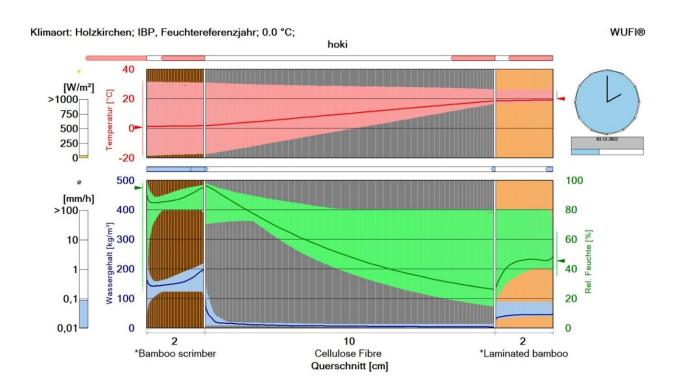
The WUFI software from Fraunhofer IBP shows a material's response to moisture over time by means of a film. The y axis indicates temperature and moisture content, while the x axis shows a cross-section of the component. Credit: Fraunhofer-Gesellschaft
