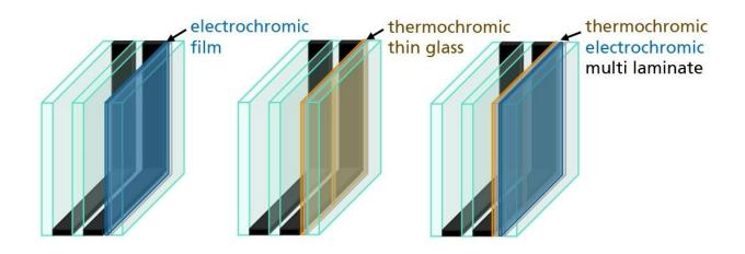
The structure of a window with Switch2Save technology: versions with electrochromic or thermochromic coating are possible, as well as a combination of the two technologies in one window. Credit: Fraunhofer-Gesellschaft
