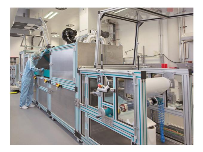
The coatings are manufactured using a roll-to-roll process. At just a few hundred micrometers thick, both the electrochromic film and the thermochromic thin glass substrate are extremely thin. Credit: Fraunhofer-Gesellschaft
