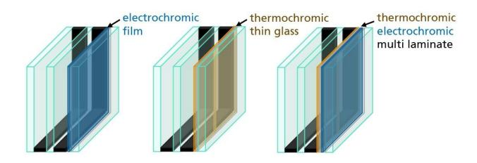
The structure of a window with Switch2Save technology: versions with electrochromic or thermochromic coating are possible, as well as a combination of the two technologies in one window. Credit: Fraunhofer-Gesellschaft
