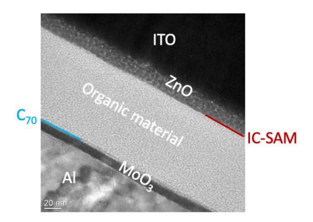
Transmission electron microscope (TEM) image of a cross-sectional slice of an OPV with the added layers of material (IC-SAM and C70) between the organic material and the external buffers, after the material was subjected to high intensity light to replicate an estimated age of 30 years. It reveals an intact organic active region with no breakdown at the edges. Credit: Kan Ding, University of Michigan
