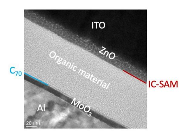
Transmission electron microscope (TEM) image of a cross-sectional slice of an OPV with the added layers of material (IC-SAM and C70) between the organic material and the external buffers, after the material was subjected to high intensity light to replicate an estimated age of 30 years. It reveals an intact organic active region with no breakdown at the edges. Credit: Kan Ding, University of Michigan
