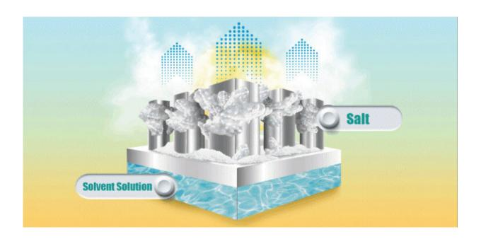
KAUST scientists have developed a simple cooling system based on solar energy and the cooling effect of saltwater evaporation that could be used for refrigeration in hot regions with limited access to electricity. Credit: KAUST; Veronica Moraru
