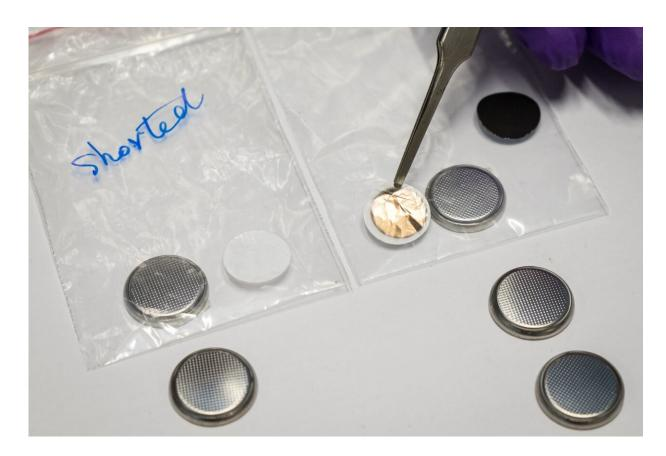
The NTU anti-short layer (upper right held by tweezer) stops short circuits from happening in li-ion batteries. Credit: NTU Singapore
