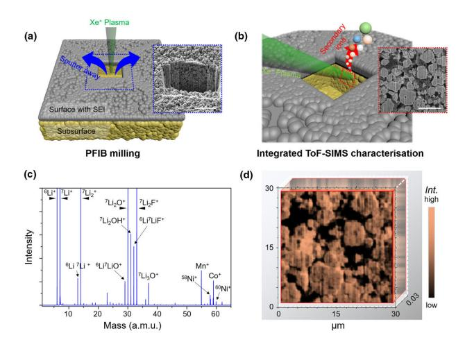
Integrated Xenon ion plasma FIB milling and ToF-SIMS technique. a) The schematic diagram of the first step Xe+ PFIB milling for the cycled NMC electrode, and the SEM image of the cross-sectional interface (inset, blue box, scale bar:  $40~\mu m$ ). (Gray layer: external surface with SEI, Yellow layer: subsurface underneath the external SEI.) b) The schematic diagram of the integrated ToF-SIMS characterization for the selected area (red box) on the cross-
