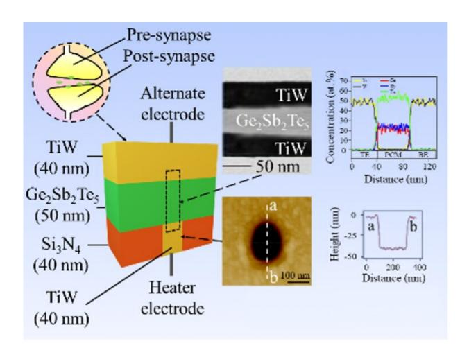
Illustration of the device structure of the phase-change artificial synapse. The heater and alternate electrodes correspond to the post-synaptic and pre-synaptic neurons, respectively. Credit: SUTD
