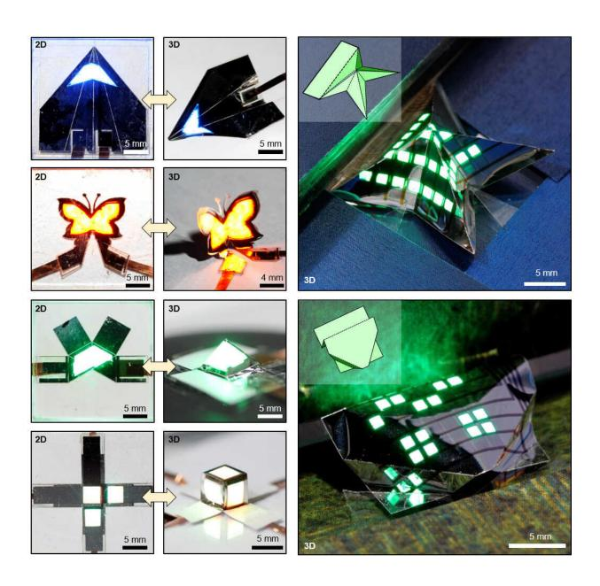
Figure 1. Fabrication of 3D foldable QLEDs that can be folded freely as paper.
