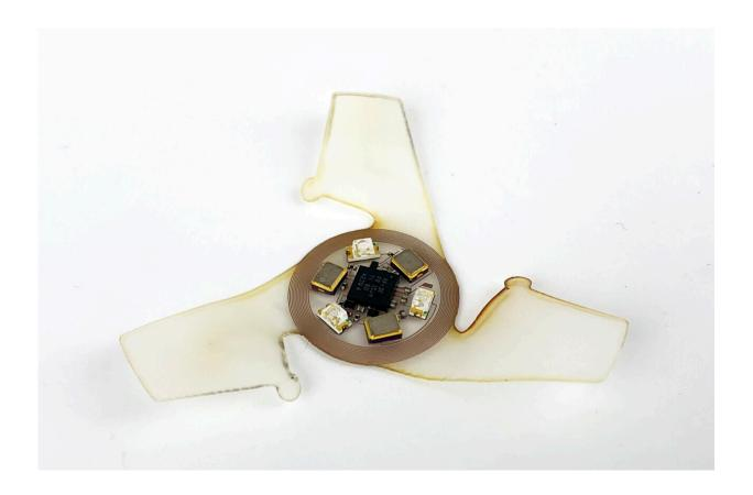
A close-up of a 3D microflier, outfitted with a coil antenna and UV sensors. Credit: Northwestern University
