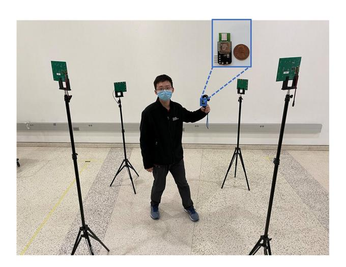
The new UWB system consists of a small electronic tag (inset shows the size of a tag compared to a U.S. penny) that transmits one signal simultaneously to four anchors. Credit: University of California - San Diego
