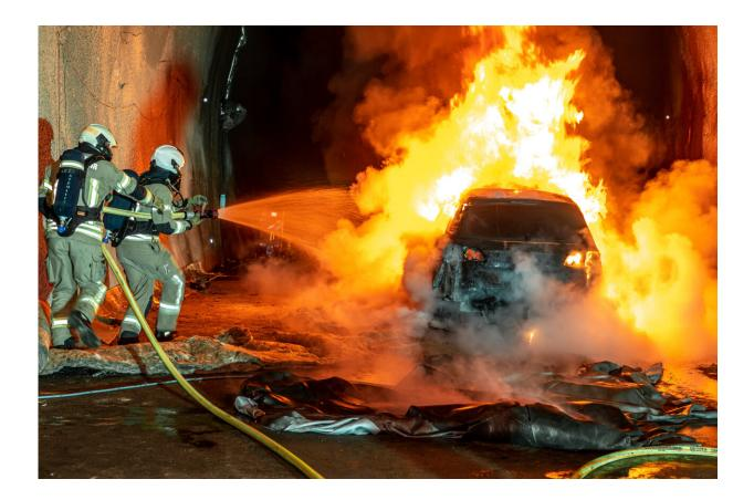
In the course of the project, the fire brigade was able to test different extinguishing methods for burning e-vehicles in tunnels. Credit: Lunghammer - TU Graz
